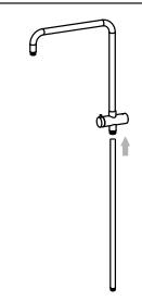
Screw bottom rail section onto diverter 5. valve.
