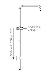
Mark down vertical between 550mm and 750mm from centre of water outlet.
