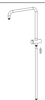
5. Screw bottom rail section onto diverter valve.
