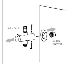
Loosen grub screws on body of diverter valve and withdraw the brass easy fit.
