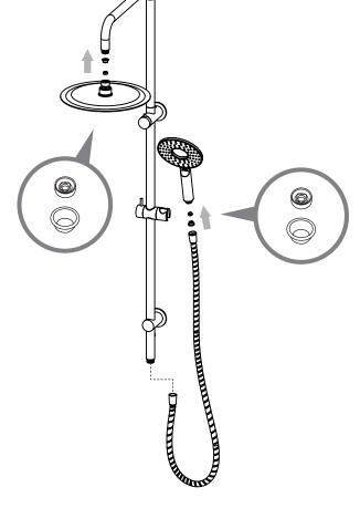
Check the flow restrictor is fitted onto the handpiece. Screw the hose onto the diverter and handpiece and attach the handpiece to
