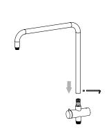
Fit overhead shower arm onto diverter valve and secure grub screw on shower arm into the **4.** white bushing.
