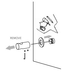
Loosen grub screws from the lower mounting bracket and remove the easy fit. Mark and use screws to fasten easy fit into place, then slide chrome flange over.
