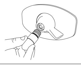
2. Screw the elbow end with the black 'o-ring' into the wallset. The plastic flange provided will not be needed for this conversion.
