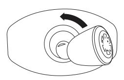
1. Remove the shower head from the existing Feltonmix wallset by gripping the shower head stem and turning it anti-clockwise.
