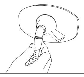
For Mains Pressure, fit flow restrictor into the handpiece first.
