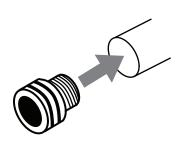
Screw the brass nipple into the wall wingback/ outlet. Sealant required on thread to achieve a 6. water tight seal. Flush out pipework.
