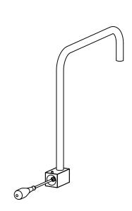
Assemble the top section by aligning the arm with the top mounting bracket.
