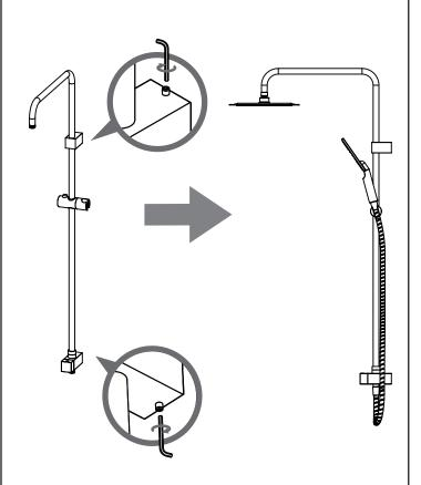
Fit the entire assembly onto wall by tightening the grub screws on the bottom and top mounting bracket.
