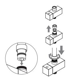
Fit the centre rail to the bottom bracket by un-screwing the thread and inserting the rail into the bottom bracket. Re-assemble the existing layout as shown and tighten to **3.** lock into place.
